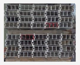
Pictured on the left is a pack of 51 secondary beams over three rows of 17. In between each row of beams is a small ply rip and in between each pack is a set of timber bites.
