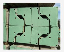
The Aluminium panels (pictured on the left) are placed on top of each other. The bottom most panel is placed face down and all subsequent panels on top of this are placed face up. Panels are stacked in packs of 10 and bound together by 2 crimped steel bands.
