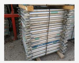
The ledger frames (pictured on the right), are stacked in packs of 25 and banded together with a single steel band. While the outer legs (pictured in the centre), are stacked end to end in packs of 45; 5 rows of 9, then separated with timber bites and held together with 2 crimped steel bands.
