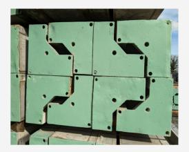
The steel panels (pictured on the left) are placed on top of each other. The bottom most panel is placed face down and all subsequent panels on top of this are placed face up. Panels are stacked in packs of 8 and bound together by 2 crimped steel bands (pictured in the centre).
